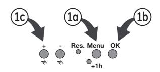
Should the OFF command be the same day of ON command then select **Menu** to terminate programming or select **OK** to go to a new program ON setting.
