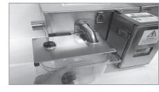
Empty collection container into barrel. This can then be taken away by a local rendering company for recycling.
