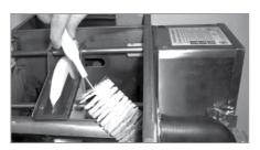
Use a bottle brush to clear grease deposits from the trough and inside of pipe
